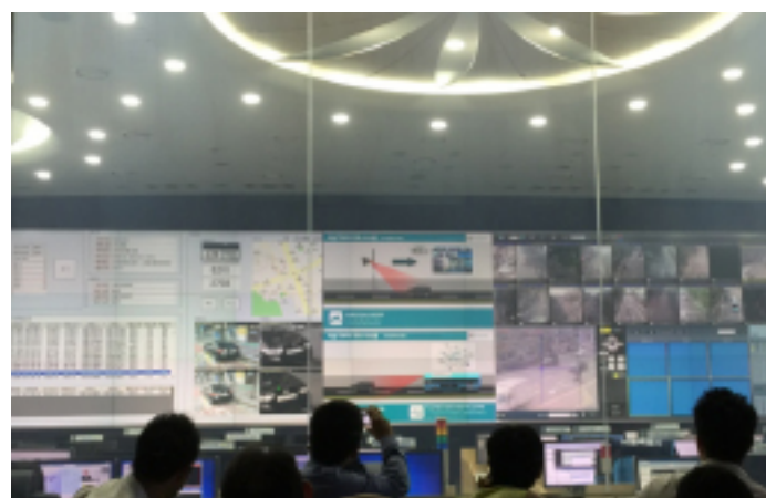
Use of CCTVs in TOPIS system for real-time monitoring of the transportation network in Seoul City
