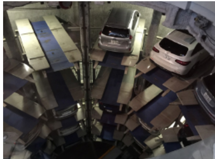
Underground car parking system to free up space above ground for other uses
